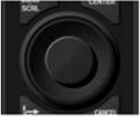
The large rotary knob offers a friendly operation for zoom in/out like you rotate the RotoKey™ of TZT9/14/BB. The big joystick makes it easier to move a cursor. With the TZTL12F/15F v3.01, pushing the joystick selects the highlighted items in contextual menus, settings, Layer, etc.
